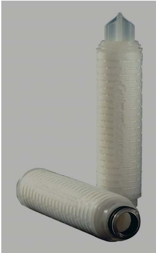
**HyperGuard** cartridge is a filter specifically designed for reduction of bioburden and particulate levels to protect final 0.1 and 0.2  $\mu\text{m}$  system filters. The pleated filter medium is modified polyethersulfone hydrophilic membrane specifically developed for rigorous operating conditions in many filtration applications.
